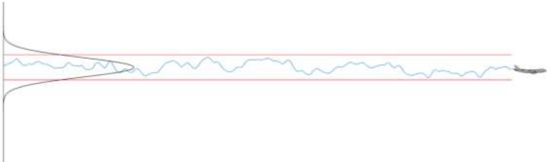
Figure 36 Sample path for vertical trajectory of an aircraft (axes not to scale).
