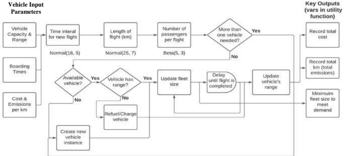
Figure 2. Operational Transportation Simulation used to compute Fleet size, Costs and Emissions
