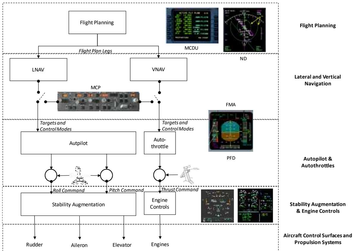
Fig. 1: Stack architecture of the modern airliner flight deck automation functions
