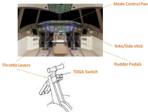
Fig. 2: Example of Input Control Devices: Mode Control Panel, Yoke, Rudder Pedals, Throttle Lever and Takeoff/Go Around Switch
