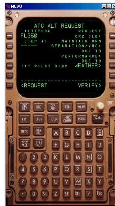
Figure 2: CPDLC - Message Received by Pilot from ATC
