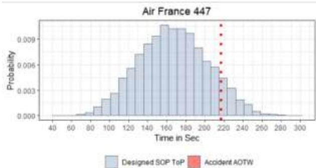
**Figure 11. Results of the Air France 447 Stall Recovery SOP AD Simulation**
