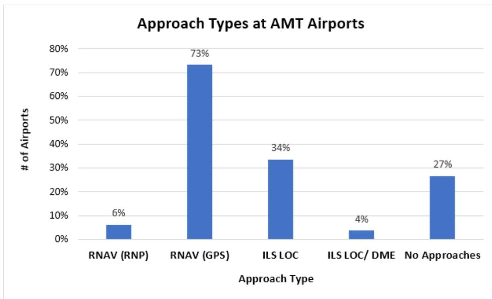
**FIGURE 10: RNAV Approaches at the airports that visited by AMT fixed-wing flights**
