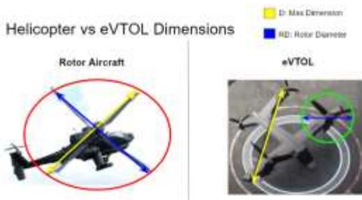
Figure 9. Helicopter vs eVTOL Dimensions
