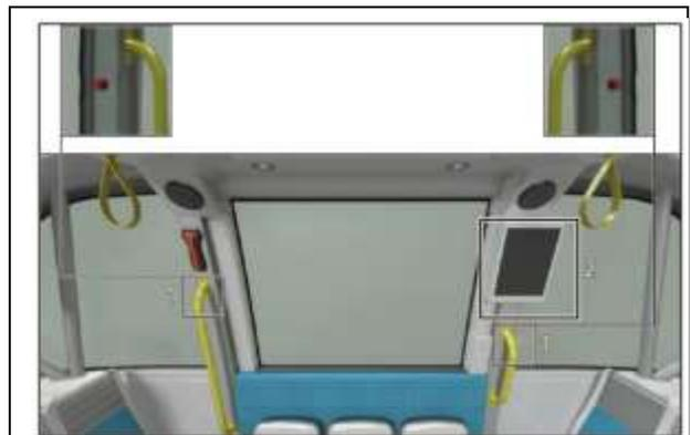
**FIGURE 2: On long-side opposite door: (1) red emergency stop buttons (inset 1), (2) information display screen located (inset 2).**
