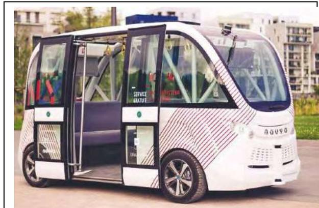
**FIGURE 1: Shuttle bus involved in the collision. Passenger entry/exit through sliding side door. Seating for 11 and standing room for 4. Can operate in either direction forward/backward.**
