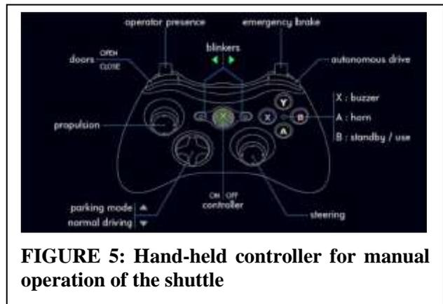
**FIGURE 5: Hand-held controller for manual operation of the shuttle**
