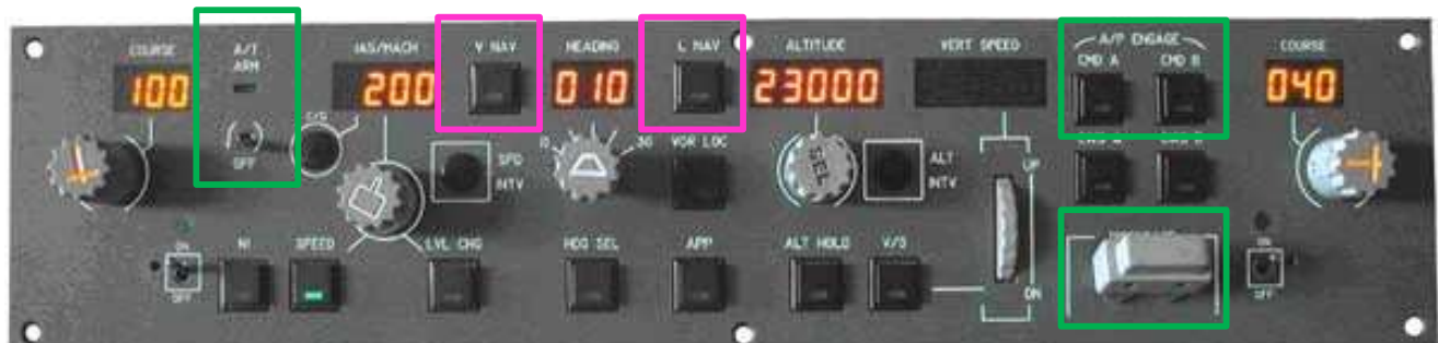
FIGURE 3: Example of Mode Control Panel (MCP) that hides the “stack” architecture with LNAV and VNAV buttons at the same “level” as mode buttons and A/T and A/P engagement switches.
