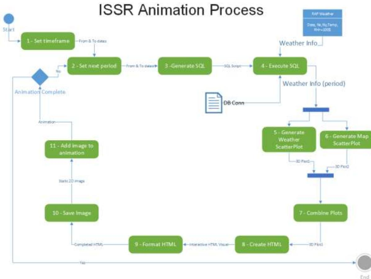
Figure 5: Process for generating ISSR 3-D visualization
