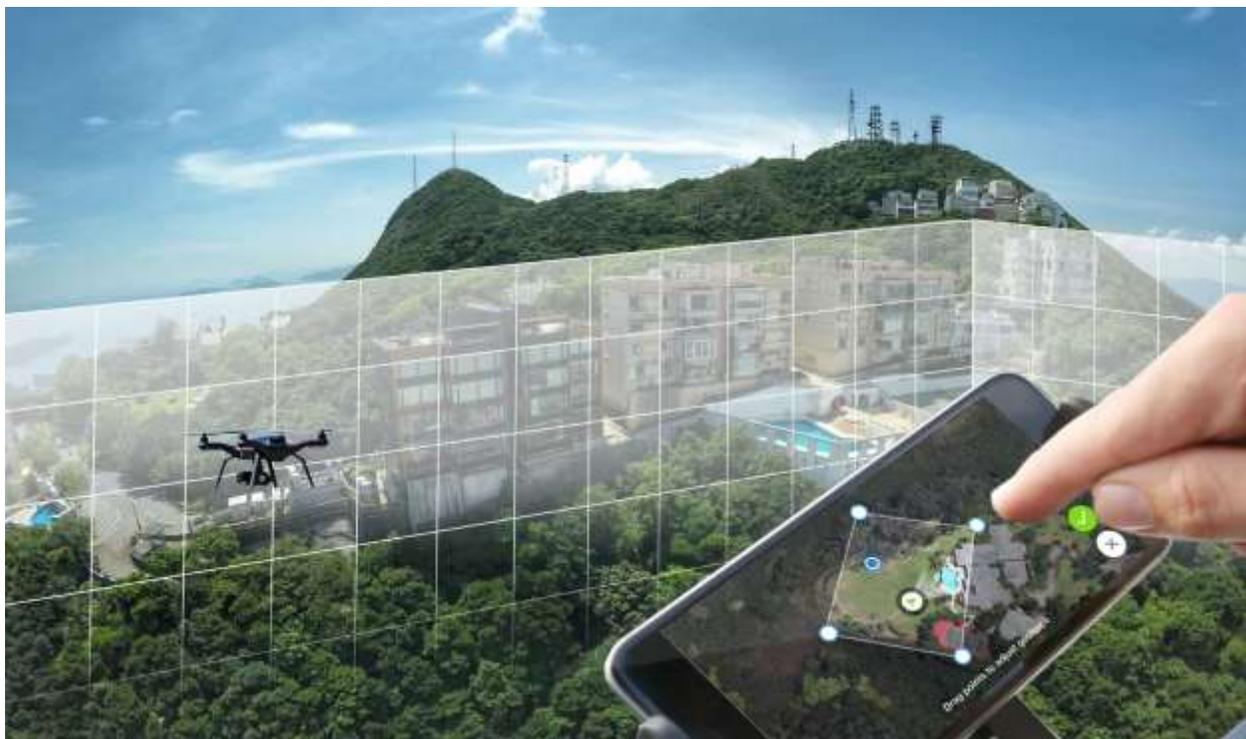
**FIGURE 3: Geofence marks a perimeter beyond which the vehicle avionics will not command the vehicle trajectory.**
