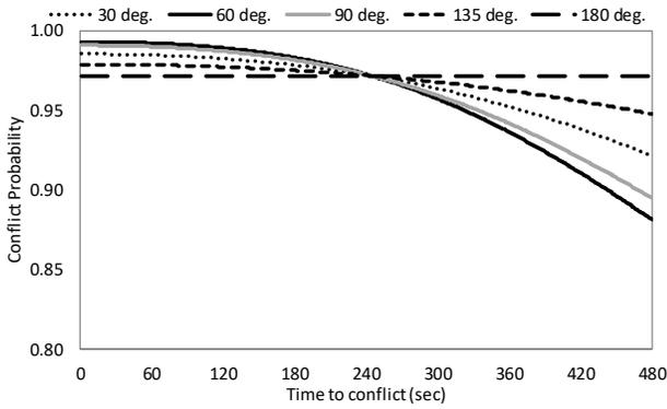
**Figure 7. Loss of separation probabilities for different path-crossing angles**
