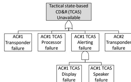
**Figure 5. Supporting fault tree for tactical state-based CD&R system (TCAS, manned)**
