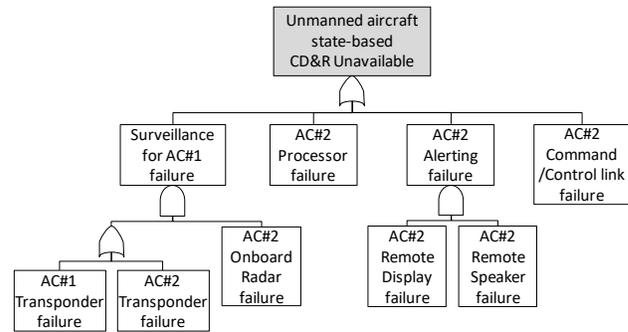
**Figure 13. Supporting fault tree for tactical state-based CD&R system (unmanned TCAS-like)**
