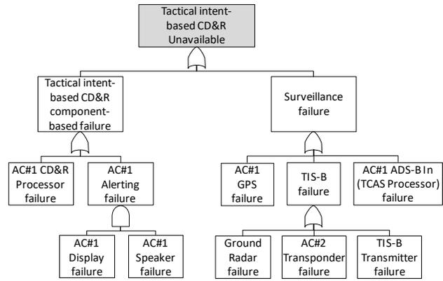
**Figure 4. Supporting fault tree for tactical intent-based CD&R system (manned)**
