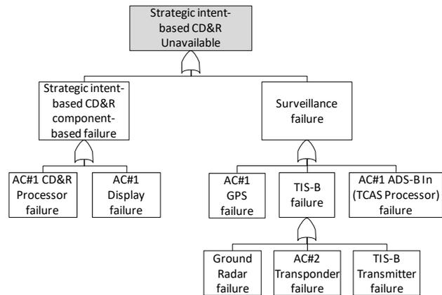
Figure 3. Supporting fault tree for strategic intent-based CD&R system (manned aircraft)
