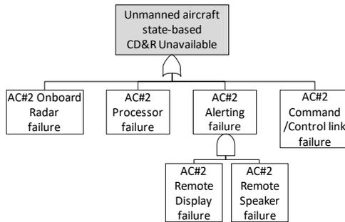
**Figure 6. Supporting fault tree for tactical state-based CD&R system (unmanned)**
