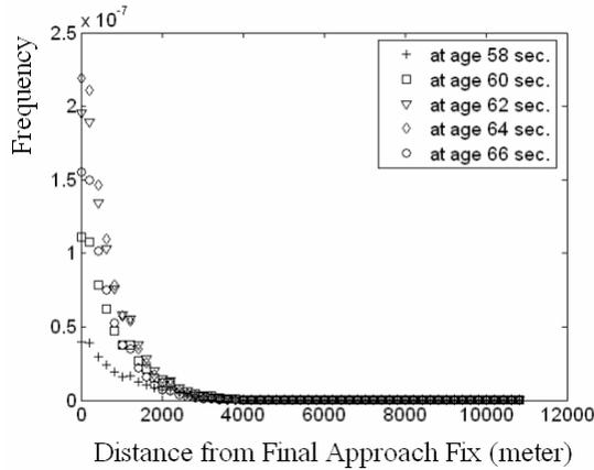
**Figure 9. Probability of Vortex Encounter at a Location When Vortex Age is close to 64 Seconds**
