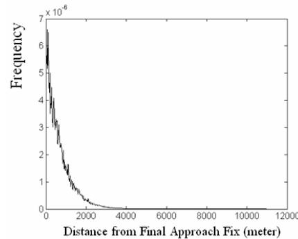
**Figure 11. Probability of An Encounter with Vortices at Age Between 40 sec. and 70 sec**
