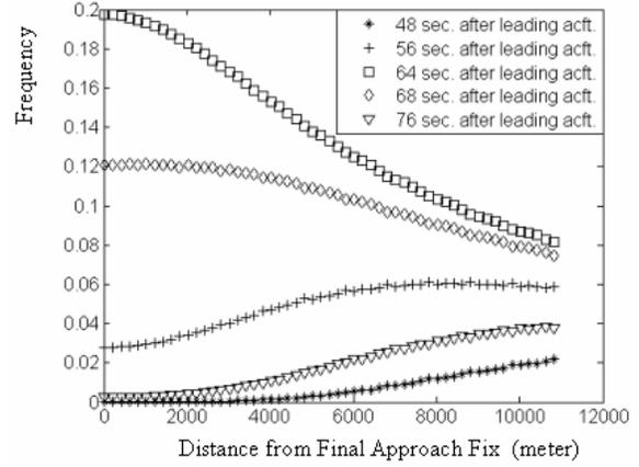
**Figure 6. Probability of Aircraft Passing A Location at Different Time**
