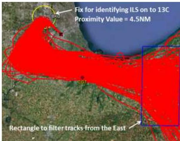
**Figure 4. Example for how Direction and Arrival Procedure is assigned to Tracks**
