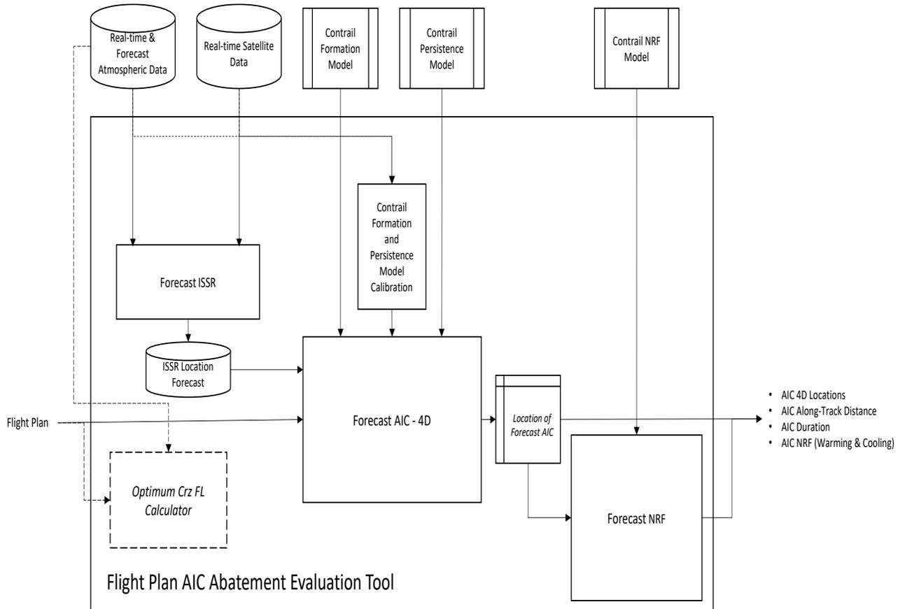
**FIGURE 4: Function Description of Flight Plan AIC Evaluation Tool**
