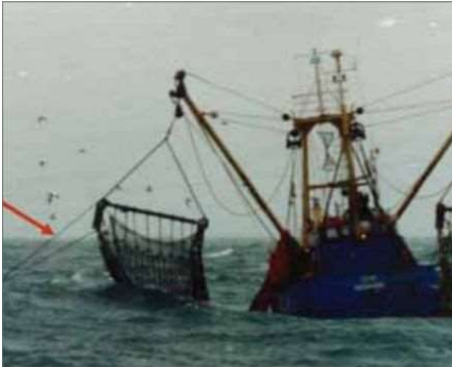
Beam trawler caught on submarine cable (red arrow) [10]
