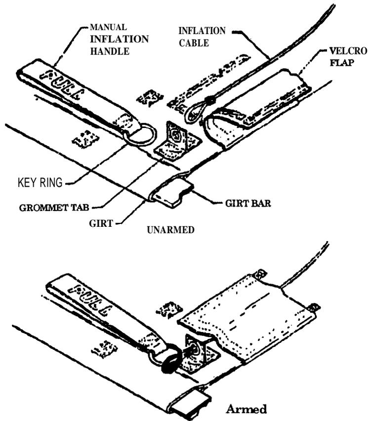
Figure 6.--Revised instruction diagram for rigging the inflation cable,
