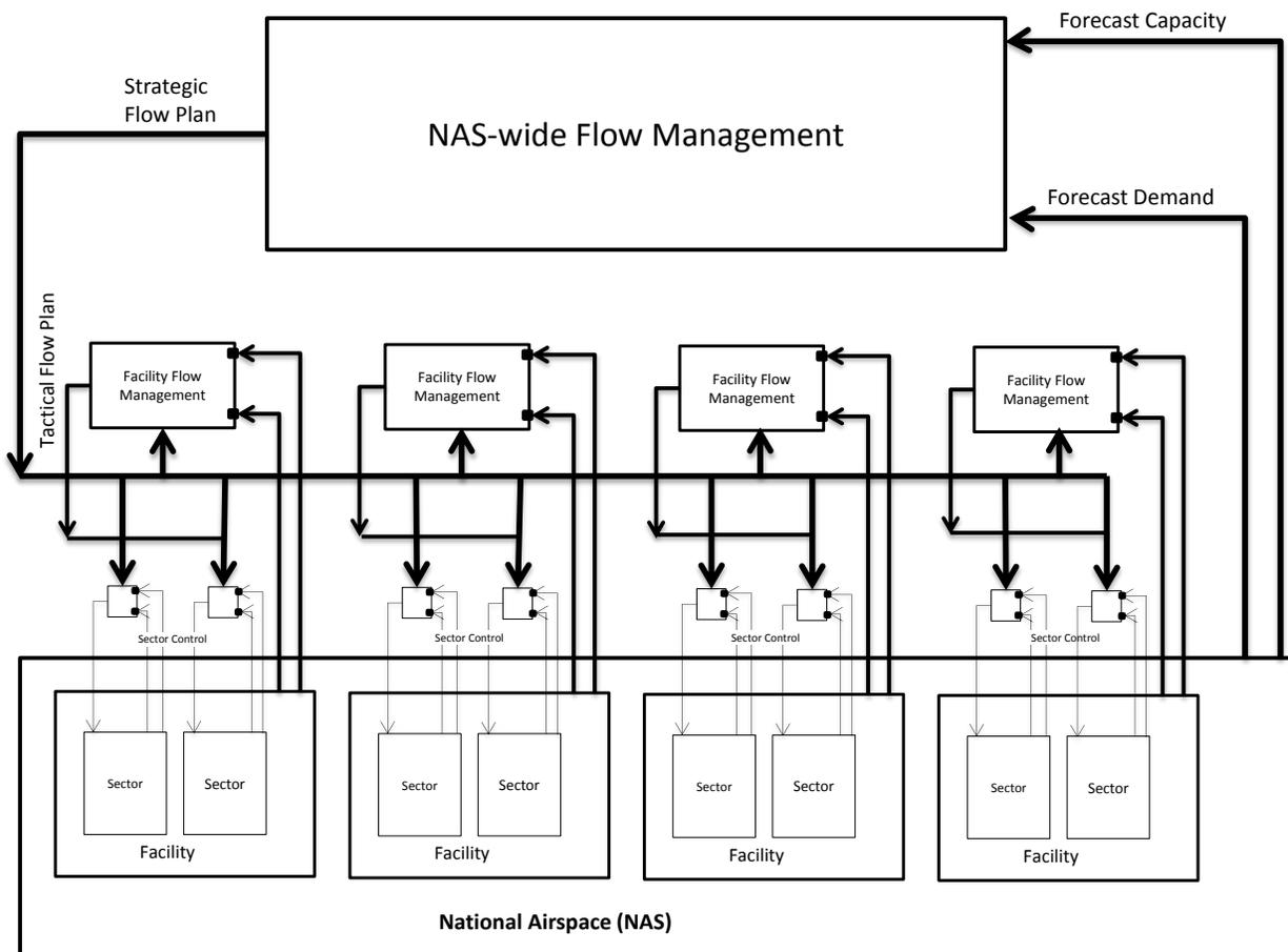
*Modern ANS function is broken down into three nested closed-loop control systems: (1) system-wide, strategic flow management, (2) regional, tactical flow adjustment, and (3) instantaneous flight trajectory control*
