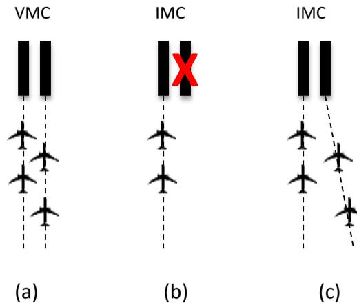
*Arrival capacity is reduced from VMC conditions with independent runway operations (a) to dependent runway operations in IMC (b). new technologies could enable an alternate procedure for IMC that allows all weather conditions on both runways (c).*
