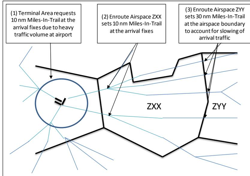
*Example of application of Miles-In-Trail restrictions to manage excessive volume of arrivals in Terminal Area can result in a ripple of MIT restrictions.*
