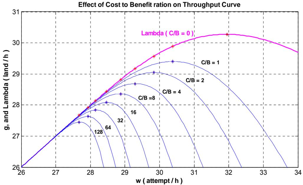
**Figure 5.5.  $g(\omega;C/B)$  of 4nmi Pairs For  $C/B = 0, 1, 2, \dots, 128$ ; WV effect included**
