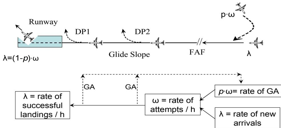
Figure 5.1. Go-around procedures on the glide slope
