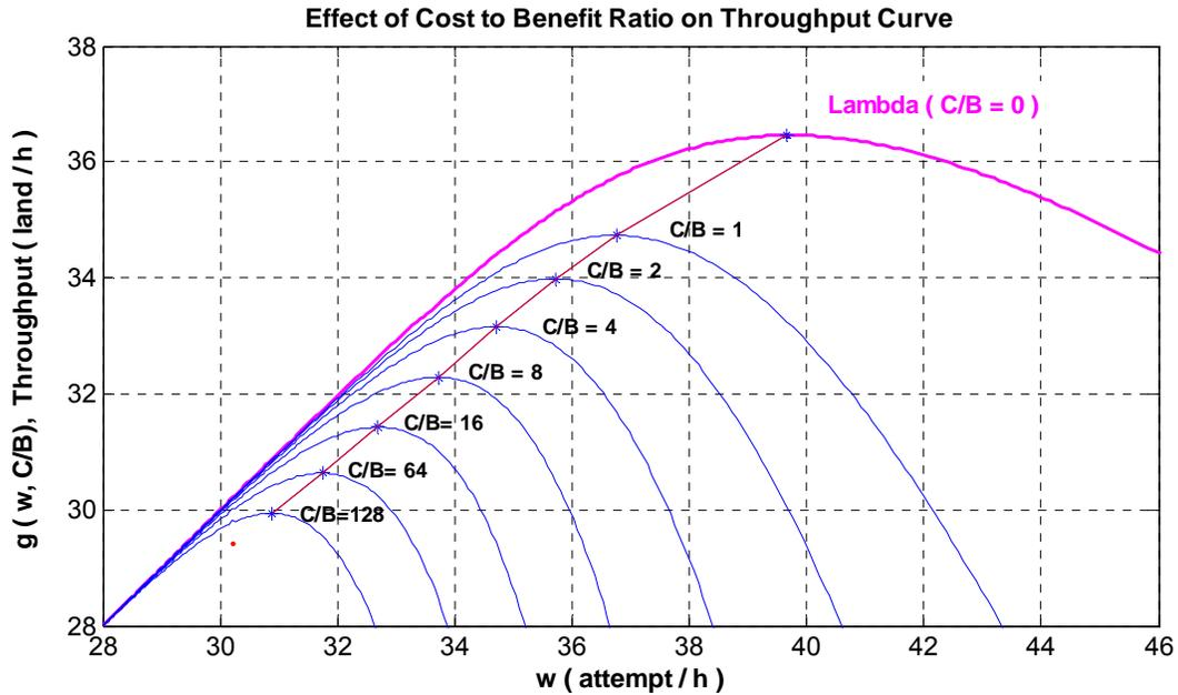
**Figure 5.4.  $g(\omega; C/B)$  of 3nm Pairs for  $C/B = 0, 1, 2, \dots, 128$ ; WV effect included**
