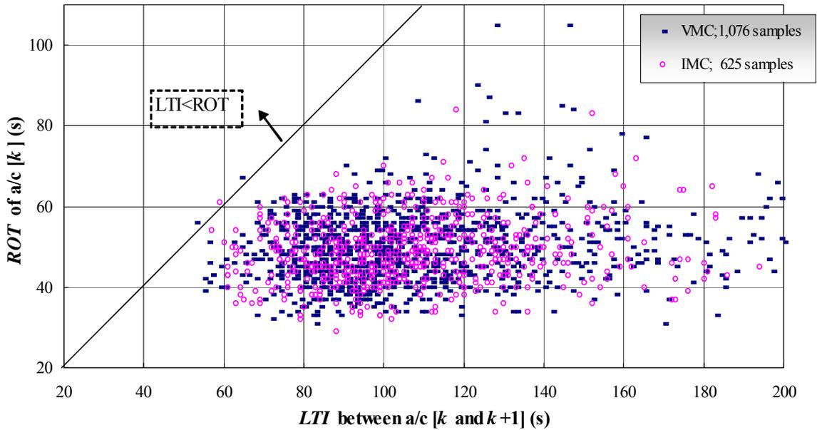
**Figure 3.10. ROT of aircraft  $k$  versus LTI between aircraft  $k$  and  $k+1$ ; Feb 2003 data**
