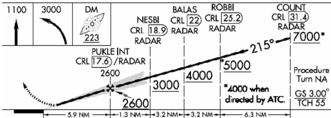
Figure 4.2. A typical final approach process
