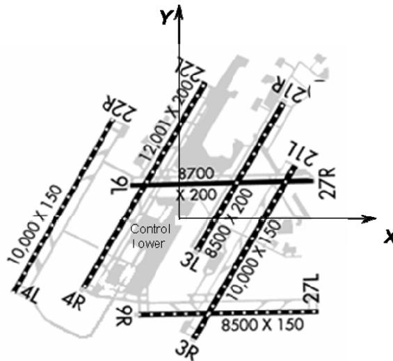
**Figure 3.1. Simplified DTW airport diagram (FAA 2006)**
