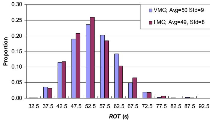
**Figure 3.9. *ROT* under VMC (895 samples) vs. IMC (590 samples); Feb 2003 data**
