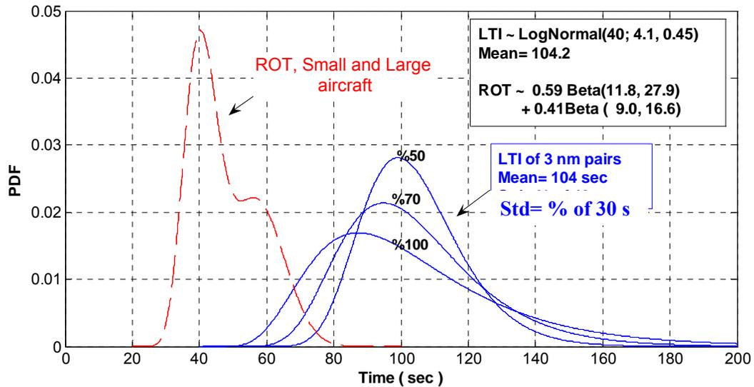
**Figure 4.7. Effect of reduced separation variance (or Std) on the overlap of *ROT* and *LTI*;  $P\{SRO\} = 0.007, 0.0014$  and  $0.0002$  for the 0%, 30% and 50% reduced Std, respectively**
