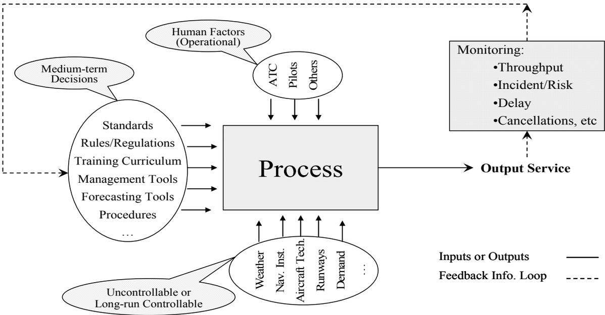
**Figure 4.1. Feedback loop on an air transportation process**
