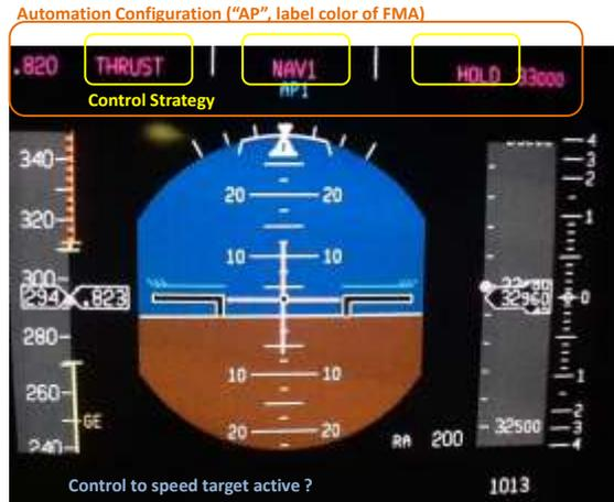
**Figure 2: Primary Flight Display (PFD) Displays Information that is an Integrated Form of Formerly Federated Gauges.**
